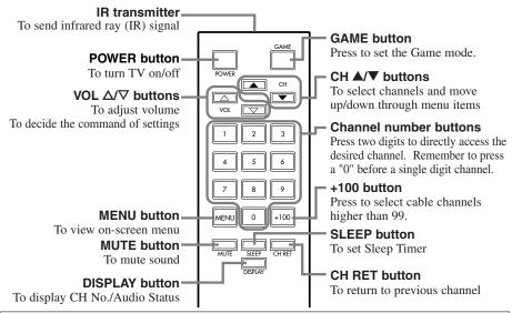
You can test if the remote control sends out the infrared signal with an AM radio. (Refer to "TROUBLESHOOTING GUIDE".)
